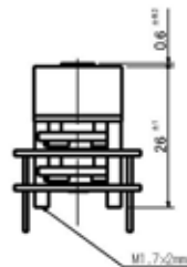
P.C.Board mounting hole detail (Viewed from mounting side)
